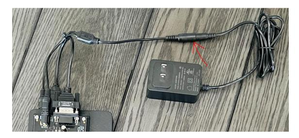
• The system is setup to automatically turn on once power is connected. You will see the power button light up once system is on, after about 1 minute the system will be fully booted up and ready to go.
